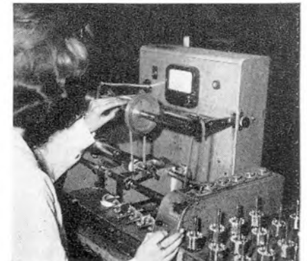
Unlike most manufacturers Ferrograph actually make their own motors on the premises. Balancing armatures is a delicate but vital job. With the help of this machine it is done speedily and efficiently
